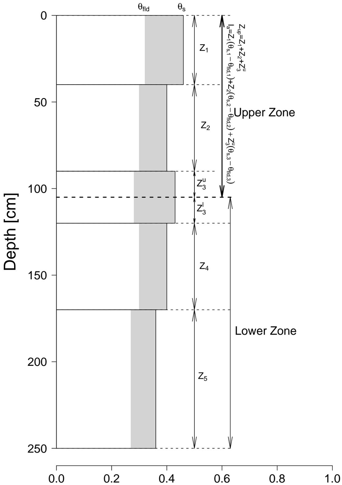
Figure 1: Schematic for the method of estimating  $Z_{up}$ .
